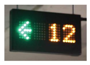
sections, counting the number of available bays in its zone. Aggregates of various areas- per lane, per floor, even per parking structure are displayed on variable message signs. The end user is guided step by step to where the available parking is located, and then directly to the green light which indicates an available space.
